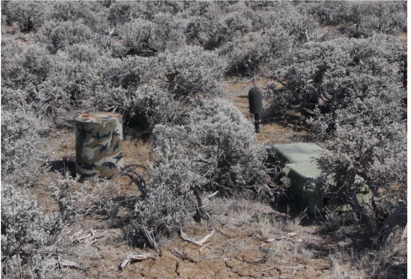
Figure 8. Data collection with LD 831 systems using two different types of windscreens, foam only and foam/fleece, both microphones 0.3 m high, 2.0 m apart.
