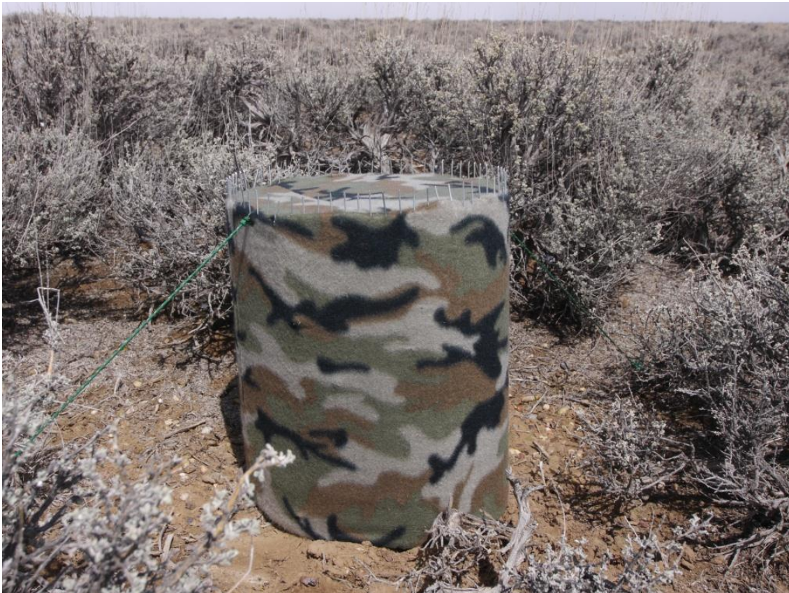
Figure 7. Windscreen made of fleece material placed over a 0.4 m (15 in) high and 0.3 m (12 in) wide wire cylindrical cage.
