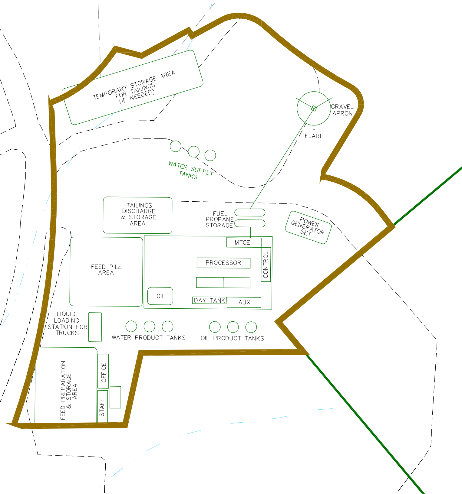
SITE LAYOUT GENERAL ARRANGEMENT PHASE 2 PROCESSING PLANT WHITE RIVER LEASE AREA, UTAH COUNTY, UTAH
