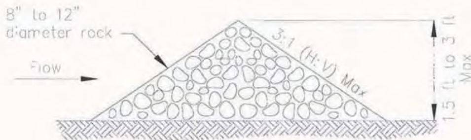
TYPICAL ROCK CHECK DAM SECTION
