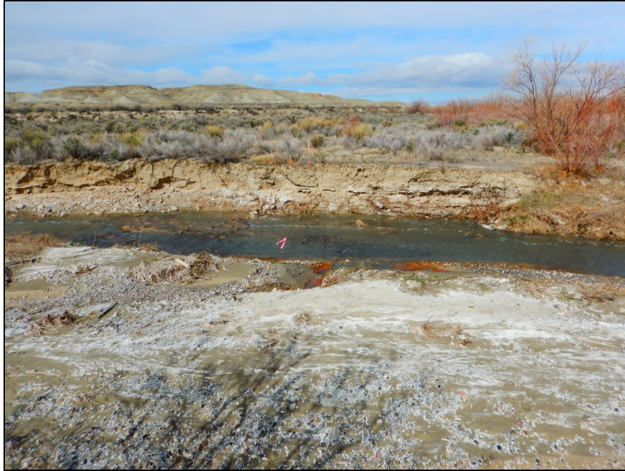
PHOTO 2.5. SITE A1 BLOCK SHEAR BANK FAILURE ON LEFT BANK AT CROSS SECTION 6
