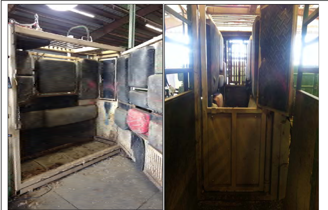
Figure II-1: The well-padded hydraulic chute at the Oregon Wild Horse Corral Facility. Note the half gate (right photo) which allows the veterinarian to safely perform the procedure.
