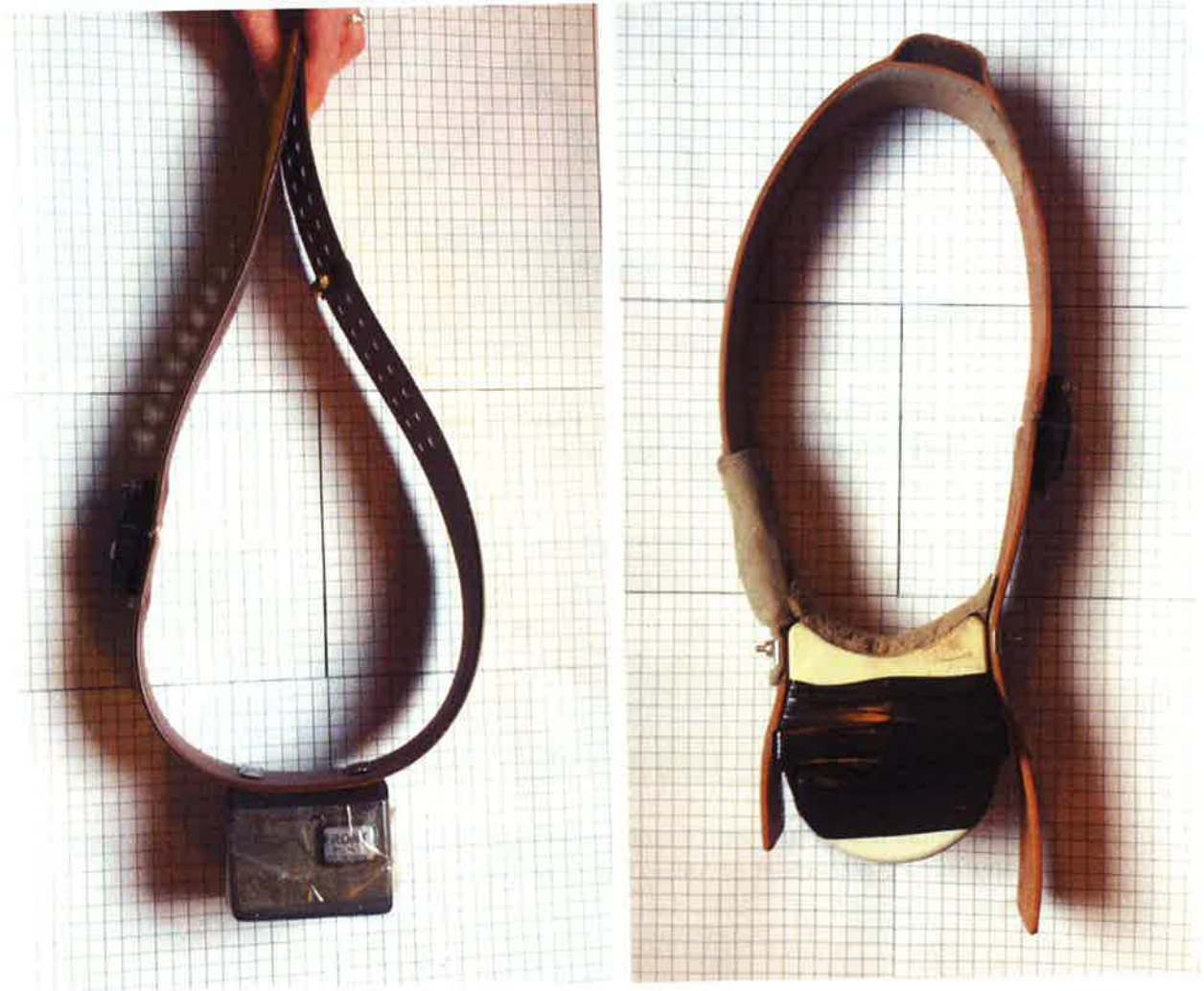
Figure 1. Two collar designs that are appropriate for wild horses and burros; one is teardrop shaped, and the other is oval shaped from Collins et al. (2014).
