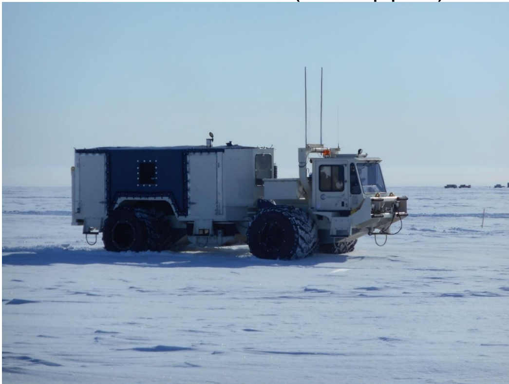
Approximately 90,000 pounds with Tracks, 60,000 with tires AHV4 Commander Vibrator (Source Equipment)
