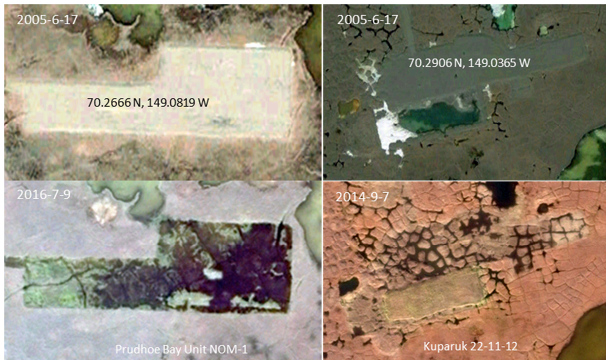
Figure 16. Thermokarst after gravel removal at exploratory well sites, which is much more prevalent than in the surrounding undisturbed tundra.
