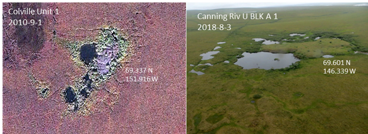
Figure 15. Satellite imagery (Google Earth) of the Colville Unit 1 exploratory well site in the NPRA drilled in 1970 (left), and aerial views of the Canning Riv U Blk A1 site (FWS photo) just west of the 1002 Area drilled in 1974 (right). Extensive thermokarst has occurred within and around the gravel pads, as well as along the bladed seismic line adjacent to the pad.
