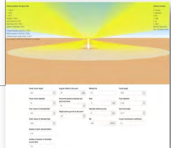
Photo and model of high-flux regions causing solar glare and avian hazards at Ivanpah Solar Electric Generating System
