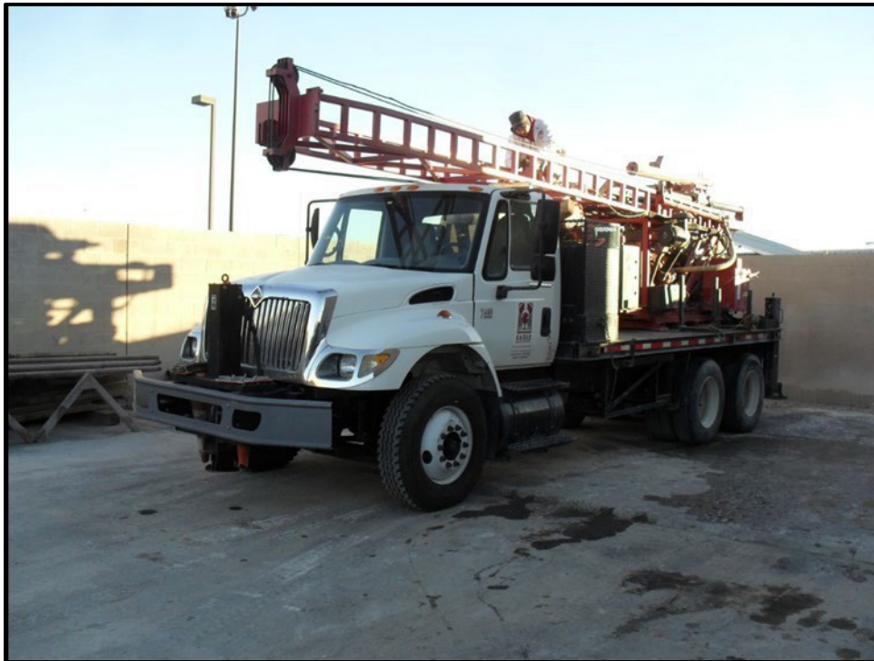
Figure 7. Truck-mounted drill rig, Diedrich D-120 type.
