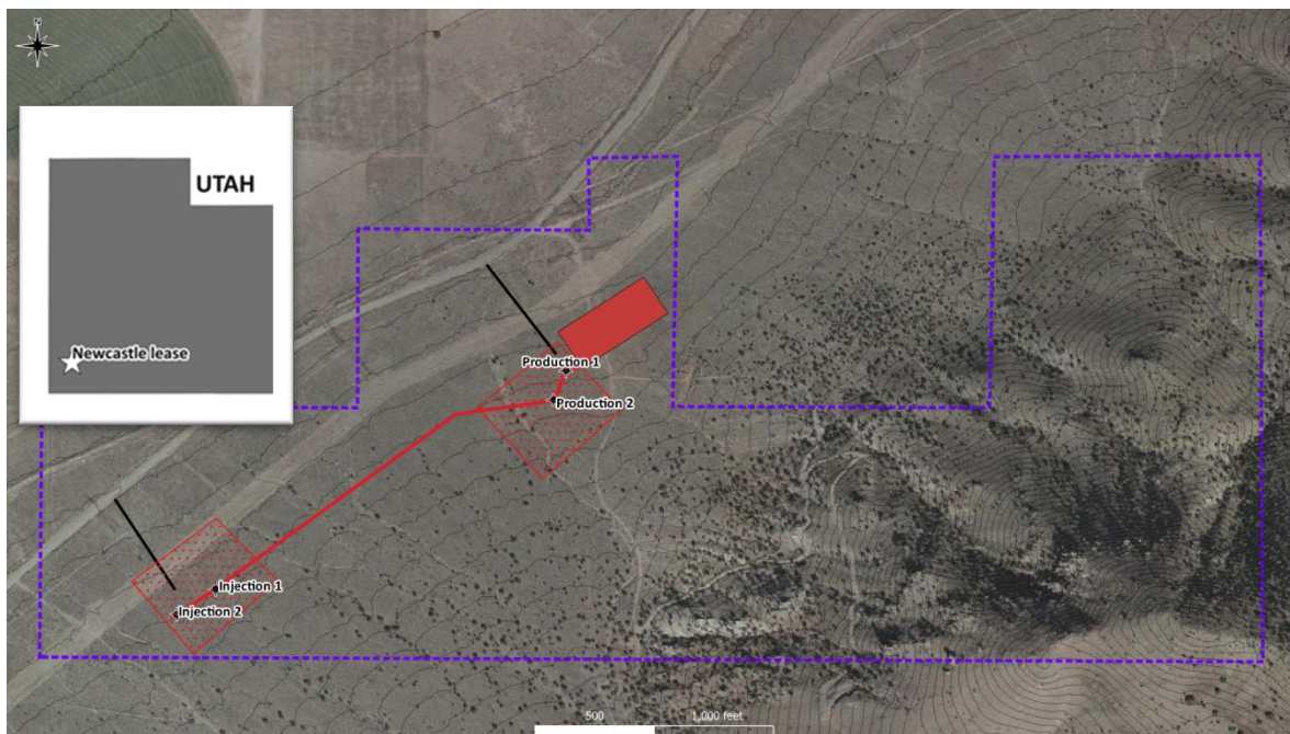
Figure 1 Project location in Newcastle, Utah with the BLM lease outline shown in purple dashed line and the geothermal plant location in a red rectangle, the injection and production well locations and the pipeline as a red line is also shown.
