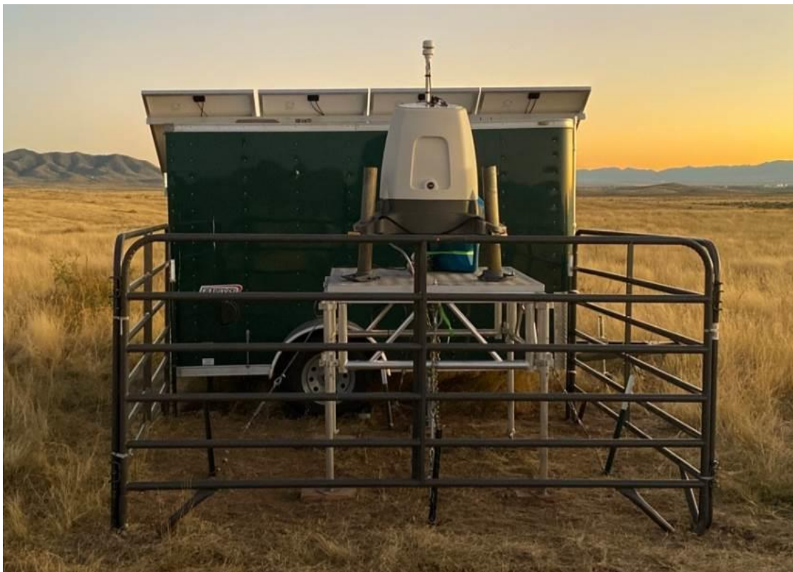
Figure 10 Remote Sensing Device (LIDAR) with Trailer and earth anchoring T-posts
