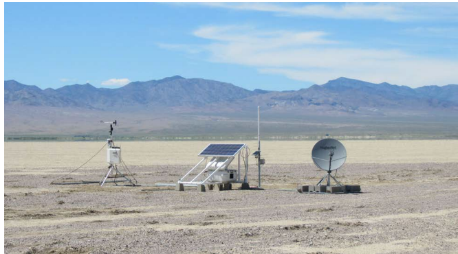
Figure 1-2. Examples of Meteorological Instruments at RRV, Including a Weather Station, Solar Panels, and Communication Dish
