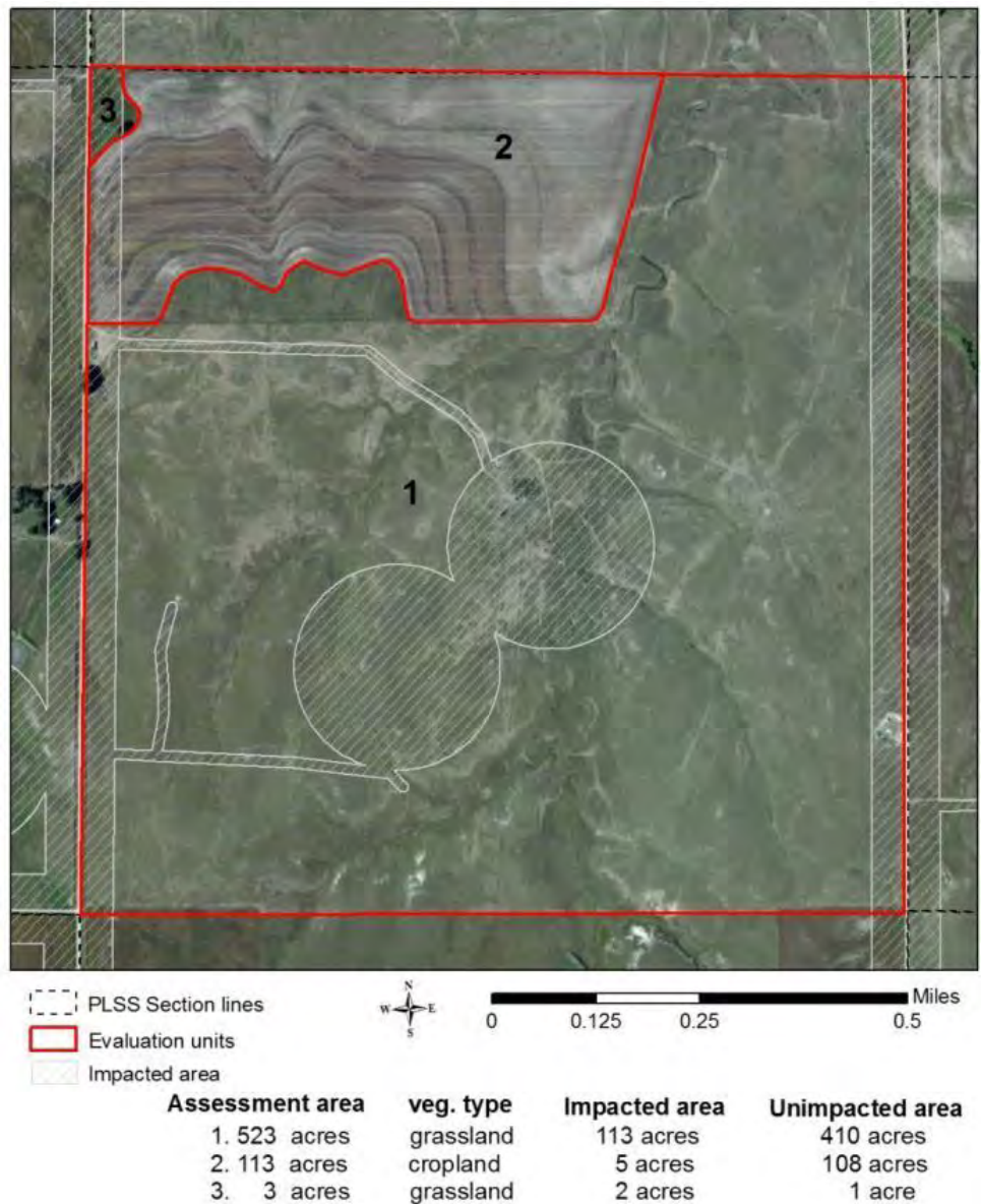
Figure H-3. Example illustrating how existing developments will be buffered to identify and quantify the previously impacted acres within the 640 acre example property where offset units are being generated. Of the 640 acres on the property, a total of 519 are unimpacted and only those acres will factor into the calculation of habitat units.
