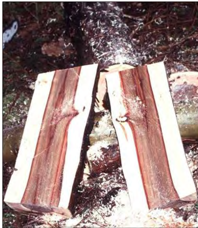
Figure 3.1. The Cambium creates a barrier zone that contains discoloration and decay in the old wood.
