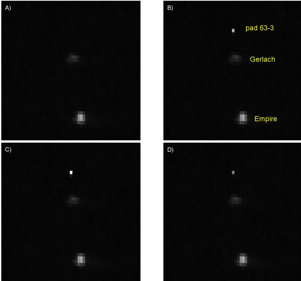
Figure 4. 15. Pad 63.3 nighttime test drill simulated VIIRS images. A) actual site in absence of drill lights (Gerlach in the center and Empire at the bottom of the images), B) expected level of lighting during active drilling, C) 1.5 times the expected level of lighting during drilling, and D) level of lighting during drilling with LED substituted lamps in mobile light plants.
