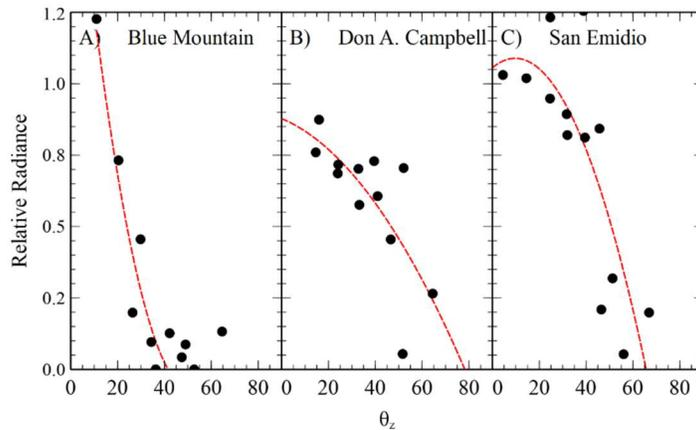
Figure 4. 12. Comparison of geothermal plant zenith angle dependency of ALAN. A) Blue Mountain geothermal plant, B) Don A. Campbell geothermal plant, and C) San Emidio geothermal plant. The relative radiance (normalized to projected zenith value) as a function of zenith angle ( $\theta_z$ ) in degrees.
