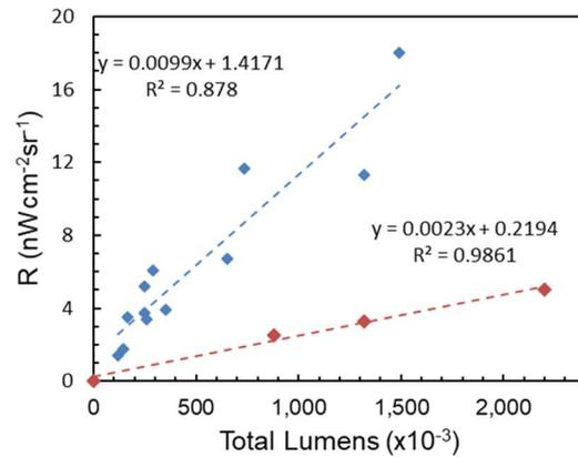
Figure 3.3. Empirical calibration of radiance observed by VIIRS radiometer. VIIRS measurements as a function of industrial mobile lighting luminance rating (nWcm<sup>-2</sup>sr<sup>-1</sup>) [3]. The blue diamonds are obtained from drill rig lighting. The red diamonds are from roadside portable light plants.
