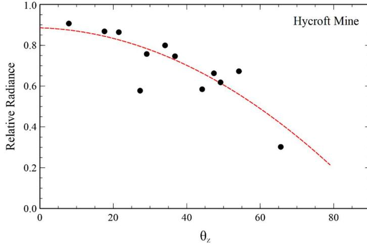
Figure 4. 13. Zenith angle dependency of ALAN at the Hycroft Mine facility. The relative radiance (normalized to projected zenith value) as a function of zenith angle ( $\theta_z$ ) in degrees.
