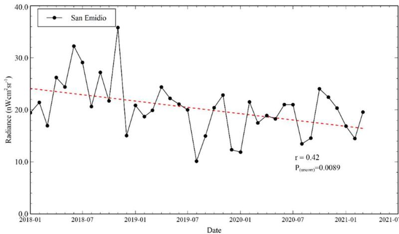
Figure 4. 8. Monthly radiance measurements at San Emidio geothermal plant.
