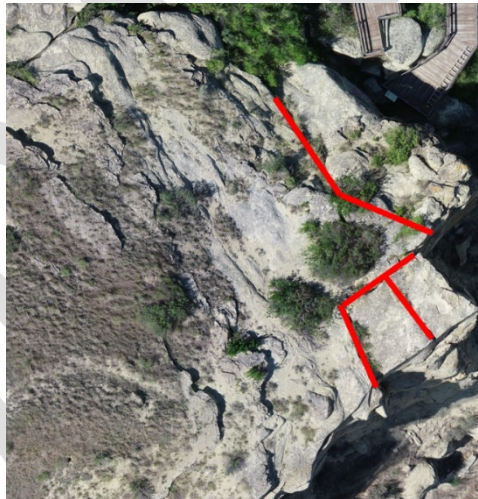
Figure 9 Major joints exposed on top of the Signature Blocks.
