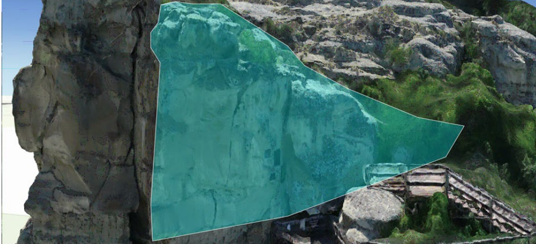
Figure 5 View of the area of analysis for scaling the Signature Blocks area.
