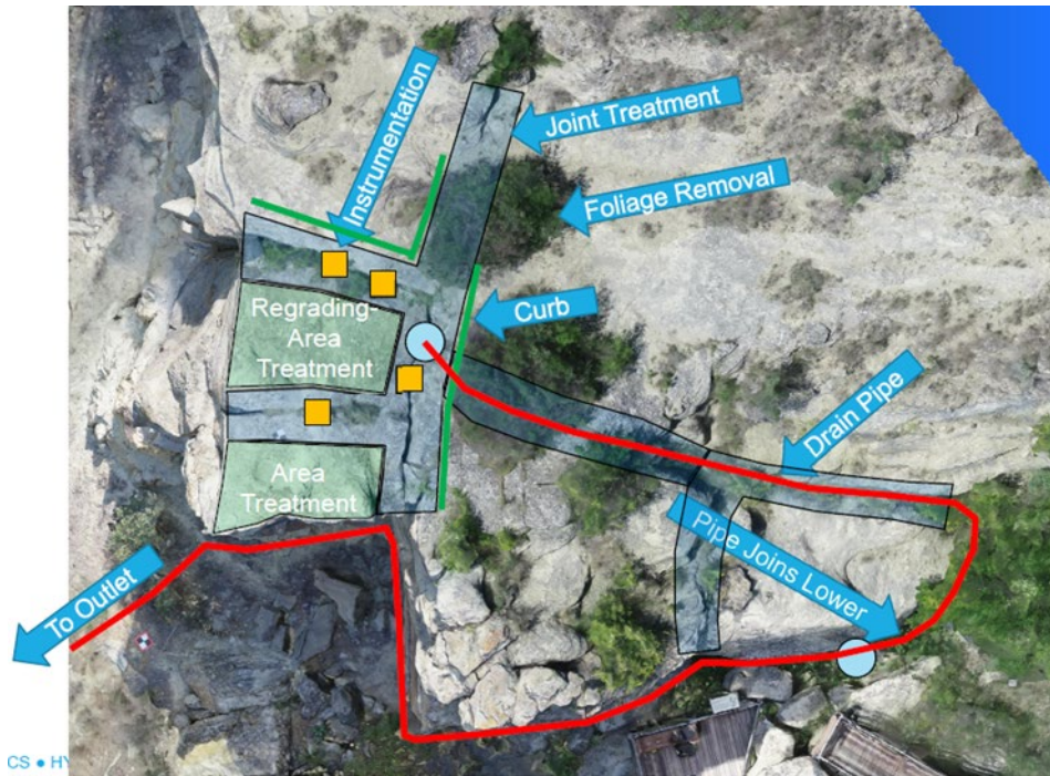
Figure 12 Possible configuration of drainage control atop the Signature Blocks to include curbing, regrading, and drainpipe.
