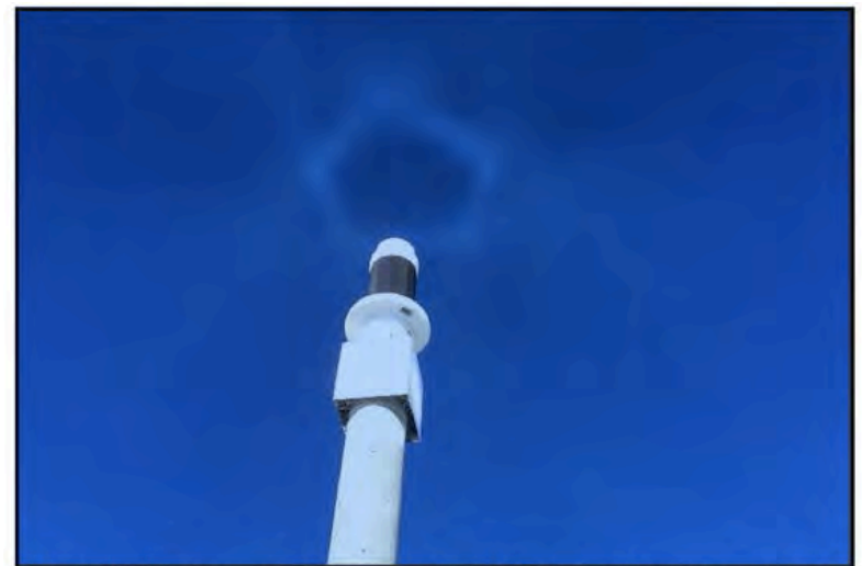
Figure 1 – The halo created by the reflected light of 3,000 heliostats which caused the bird mortalities.
