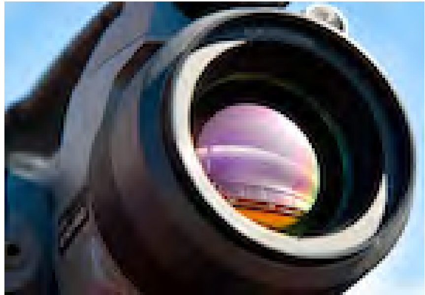
Infrared camera. Photo by Dennis Schroeder, NREL 20338
