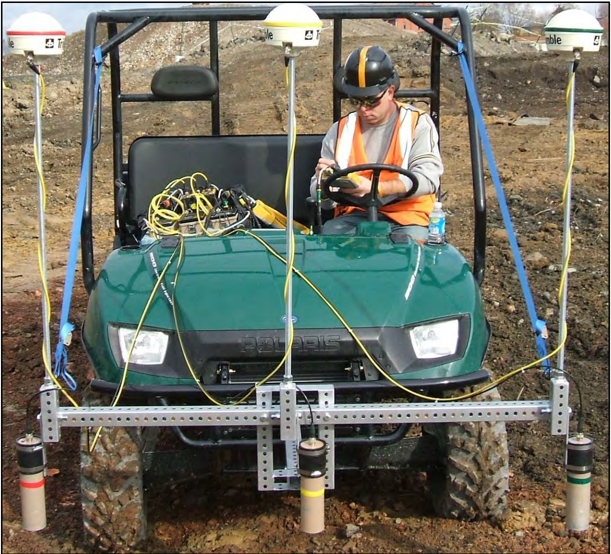
Figure 5.1-1 Example of Best Technology Available Utilized for the Roving Gamma Survey at the Dewey-Burdock Project by ERG
