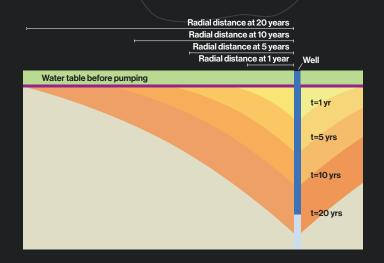
Groundwater drawdown can be predicted, butmpacts would not be fully understood until pumping commences and data is gathered over a period of years. Drawdown would be monitored at existing monitoring wells and at a set of sentinel wells at the edges of Pine Valley to make sure the predictions are accurate. The BLM would address groundwater impacts through an adaptive management plan that would detail how the project would respond to pumping effects.
