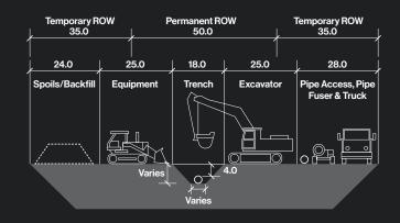
The trench depth and width would vary based on the pipe size. The pipeline would be buried with a minimum of 4 feet of cover. Pipe would be either steel or high-density polyethylene (HDPE). Typically, main lines would be steel and feeder pipelines would be HDPE. The largest pipeline size proposed is 54 inches in diameter.
