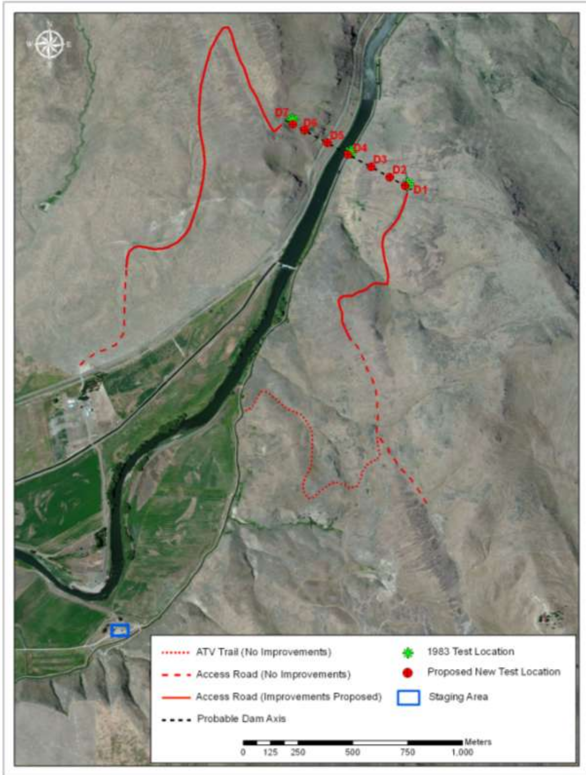
Figure 3 – Overview of site plan for geologic testing at Weiser River/Galloway dam site.
